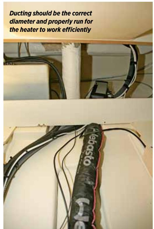
**Ducting should be the correct diameter and properly run for the heater to work efficiently**
