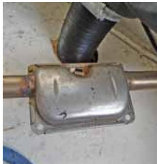
**Silencers used on vehicle heaters are not gas tight and can leak carbon monoxide inside the boat**
