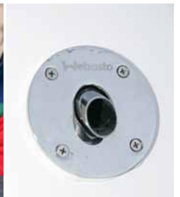
**The exhaust outlet should be fitted where the hot gas won't come in contact with fenders or dinghies. A correct exhaust outlet is insulated.**
